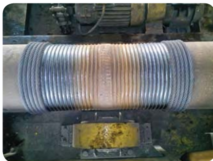
Fot. 4. Bęben suwnicy – zapas liny Photo 4. Drum in the gentry crane – supply of rope
